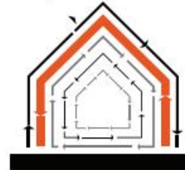
Figure 19: Stewart Brand's 'Shearing Layers' of a building
